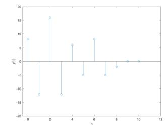
**Part** (c) Determine the response of this system to a unit impulse input; i.e., find the output y[n] = h[n] when the input is  $x[n] = \delta[n]$ . Plot h[n] as a function of n.
