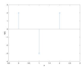
**Epilogue:** FIR filter coefficients are equal to the FIR filter impulse response. FIR filter output is the convolution of the input signal and the FIR filter impulse response (filter coefficients).
