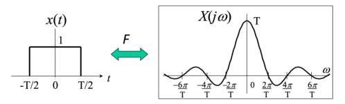
Magnitude and phase plots in MATLAB for T=1 for  $-20 < \omega < 20$  rad/s. In the magnitude response, the first zero to the right of zero frequency occurs at  $\omega = \frac{2\pi}{T} = 2\pi$ . The phase response is  $\pi$  whenever the sinc pulse goes negative.
