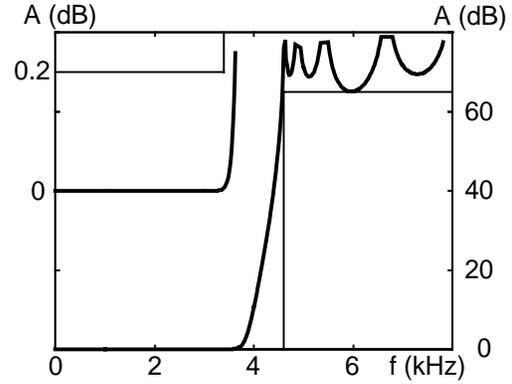
Figure 16. Attenuation of multiplierless digital IIR filter with coefficients:  $\alpha_1 = -1/2^5$ ,  $\alpha = -1/2^4$ ,  $\beta_2 = 1/2^2 + 1/2^4 - 1/2^6$ ,  $\beta_3 = 1 - 1/2^3 - 1/2^5 - 1/2^9 + 1/2^{12}$ ,  $\beta_4 = 1/2^3 - 1/2^5 - 1/2^7 - 1/2^{10}$ ,  $\beta_5 = 1/2 + 1/2^4 - 1/2^9$ ,  $\xi = 1.766$ .
