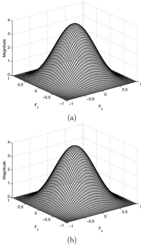
Figure 2: Frequency responses of (a) optimum product filter and (b) the product filter corresponding to the optimum compaction filter of example 1, designed using the DHT.
