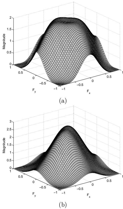
Figure 3: Frequency responses of (a) optimum product filter and (b) the product filter corresponding to the "optimum compaction filter" of example 2, designed using the DHT .
