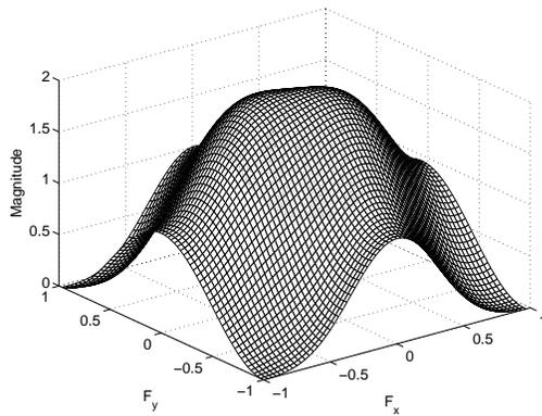
Figure 4: Frequency response of the product filter corresponding to the optimum compaction filter of example 3 designed using multi-objective optimization.
