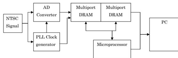
**Figure 7. Diagram of the hardware**
