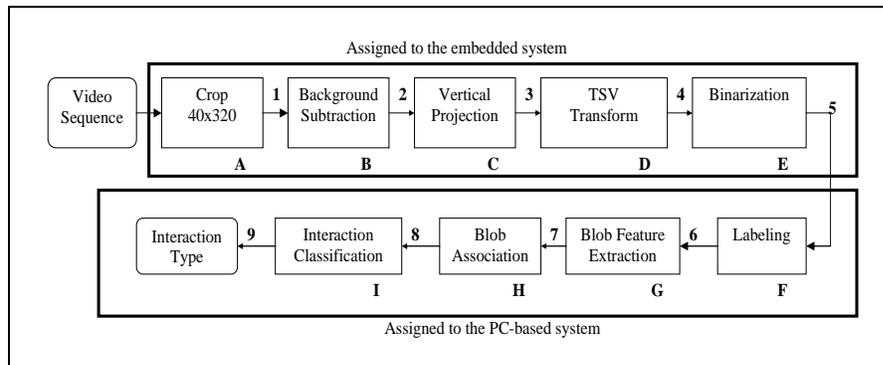
**Figure 4. Division of tasks between the embedded and PC-based system**
