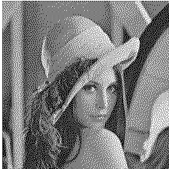
Fig. 3. Halftone generated by pixel replication induced block clustering. Here, the original image is filtered (to prevent aliasing) and downsampled. The downsampled image is then halftoned using conventional error diffusion. Pixel clustering is then induced by replicating each pixel to form a pixel-block. Note the loss of high frequency information and the blurred appearance.
