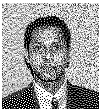
Fig. 10. Image Barcode generated using the proposed block error diffusion encoder. The rendering resolution is 120 dpi. The images may be viewed from a distance to simulate typical viewing.
