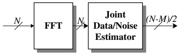
Fig. 4. A non-parametric SBL-based joint data and impulsive noise estimator in OFDM systems, using all tones. N is the FFT size, and M is twice the number of null tones.
