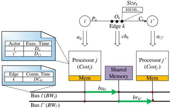
Fig. 3: Parameters and variables of the global ILP.
