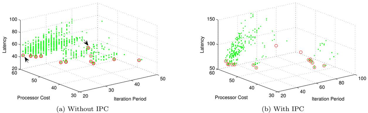
Fig. 9: Convergence to the 3D Pareto front for the MP3 decoder.
