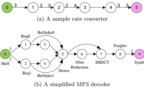
Fig. 6: The SDF models for two realistic examples.
