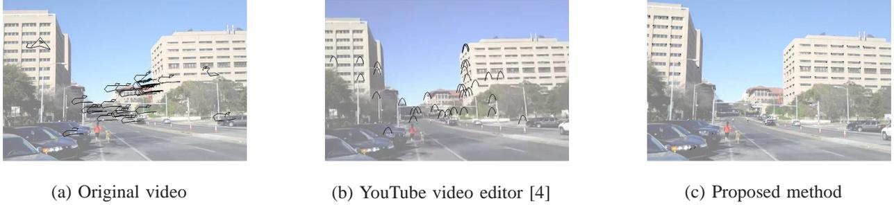
Fig. 7. Stabilization comparison for a video shot by a walking forward person. Features are tracked from frame 270 to frame 280. The feature trajectories are plotted as black curves on frame 270.
