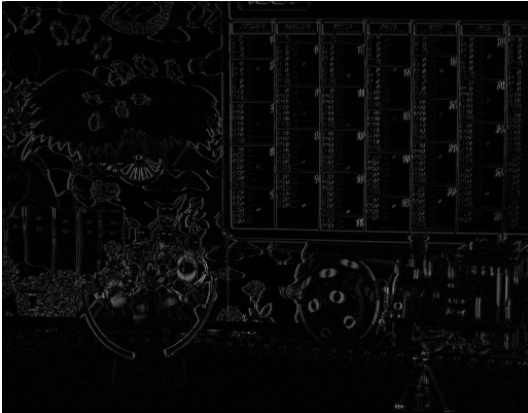
Figure 2.7: Absolute difference of frame 1 (Fig. 2.3) and frame 2 (Fig. 2.5) of the (continuous-tone) Caltrain sequence.
