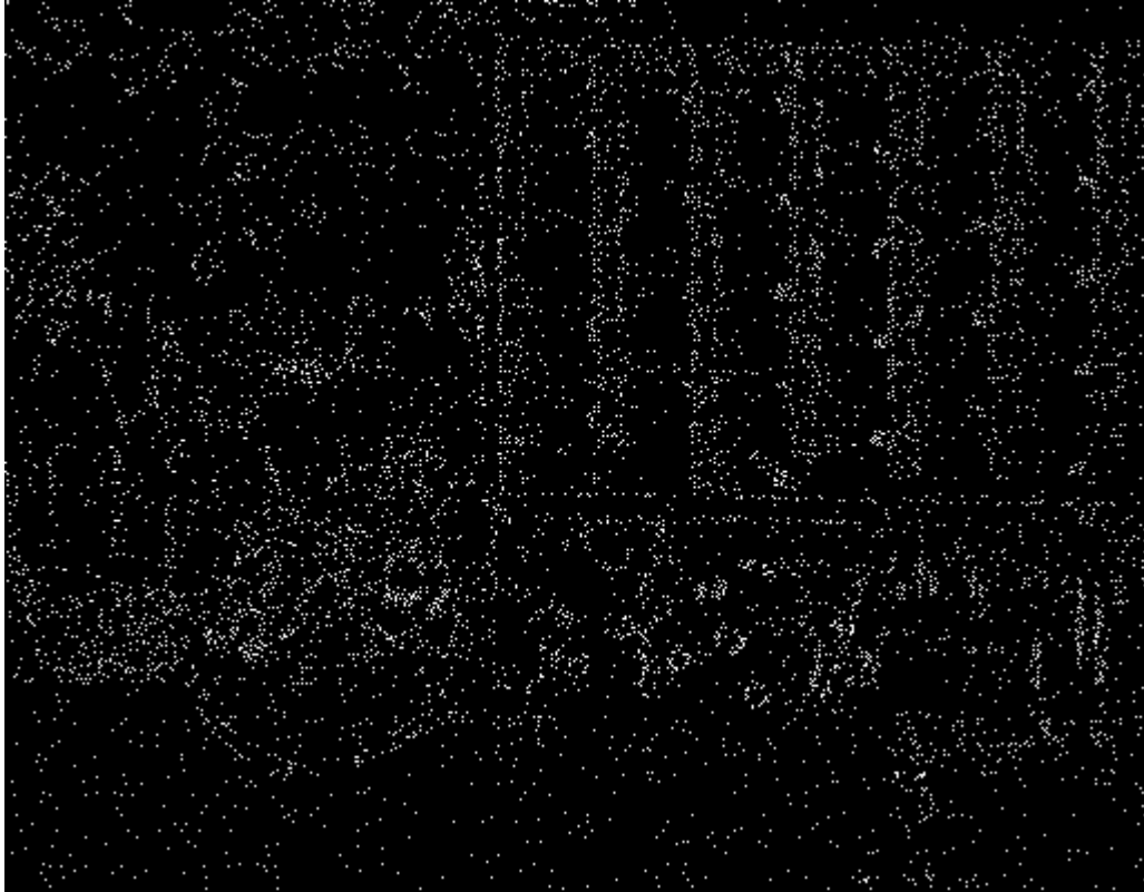
Figure 2.8: Absolute difference of frame 1 (Fig. 2.4) and frame 2 (Fig. 2.6) of the Caltrain sequence halftone. The white pixels indicate a change in halftone value (i.e. a bit flip). The Caltrain halftone frames 1 and 2 were generated using Ulichney's 32x32 void-and-cluster mask.
