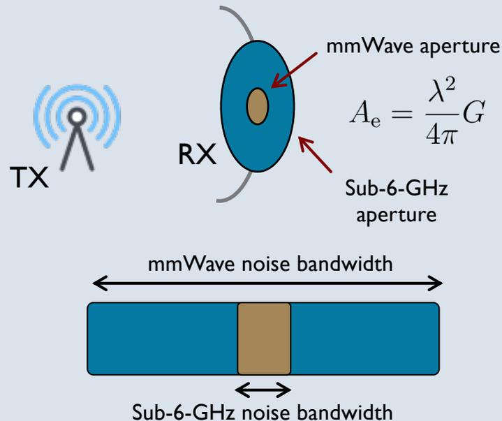
Directional beamforming is required to increase link quality through received SNR
