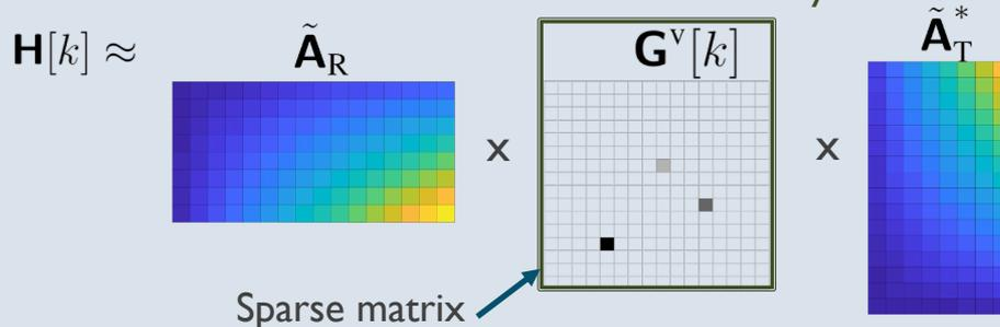
Sparse channel matrix  $\mathbf{G}^v[k]$  for 256 subcarriers, 500 MHz bandwidth, using NYUSIM channel simulator [2]
