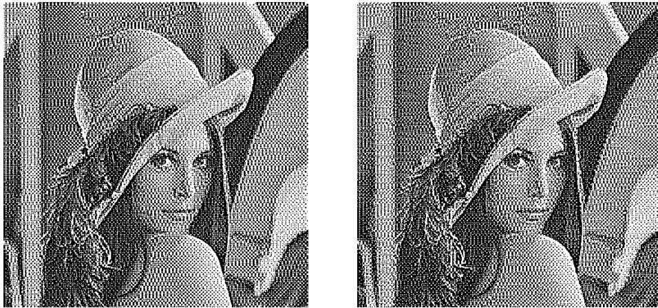
(a) AM dot modulation with array \mathbf{A} = \begin{pmatrix} 7 & 4 & 8 \\ 2 & 0 & 3 \\ 5 & 1 & 6 \end{pmatrix} (b) AM dot modulation with array \mathbf{B} = \begin{pmatrix} 5 & 7 & 4 \\ 2 & 3 & 8 \\ 0 & 1 & 6 \end{pmatrix}
