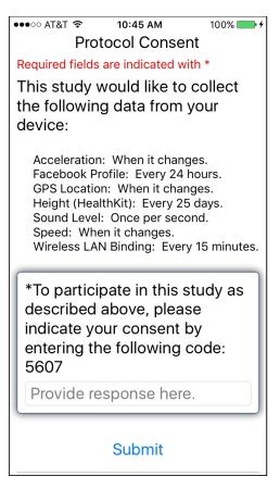
Figure 6: Upon receipt of a protocol file, the participant copies it into the Sensus mobile runtime and proceeds through a consent screen showing a data collection schedule.
