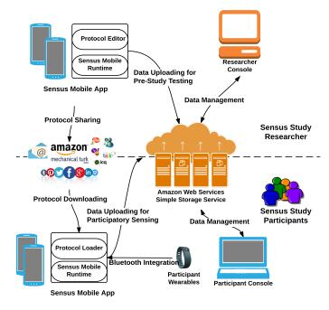
Figure 2: High-level design of Sensus.
