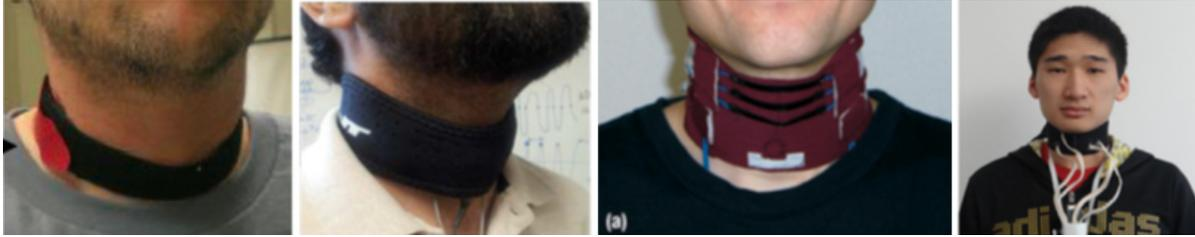
Fig. 1. Several instrumented neckbands aimed at chewing and swallowing detection have been developed over the years but their size, form factor, and aesthetic have limited their mainstream adoption. [3, 12, 17, 26]
