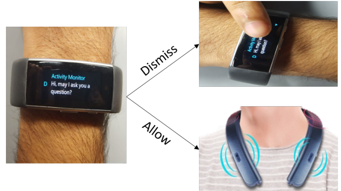
Fig. 1: Our interface requires a wearable speaker for audio input and output, and a wristband which can be optionally used to block incoming EMA prompts.
