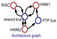
V<sub>A</sub> consists of functional resources V<sub>A</sub><sup>f</sup> (RISC, ASIC) and bus resources V<sub>A</sub><sup>c</sup>. These components are potentially allocatable.
