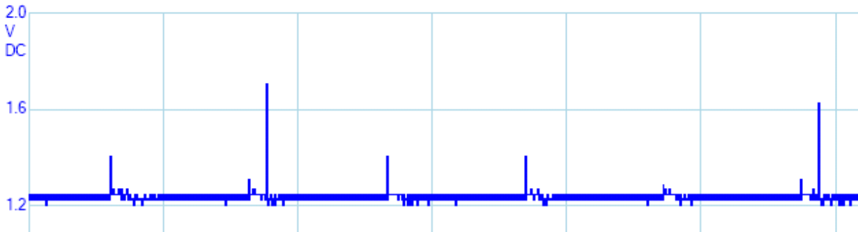
Figure 6.3. GPY0A21YK sensor output, distance=20 cm, DC mode, voltage scale is 0.4 V and time scale is 1 ms.
