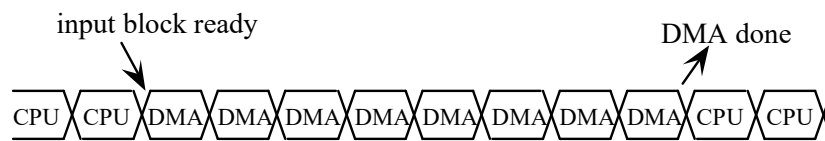
Figure 6.6. An input block is transferred all at once during burst mode DMA.
