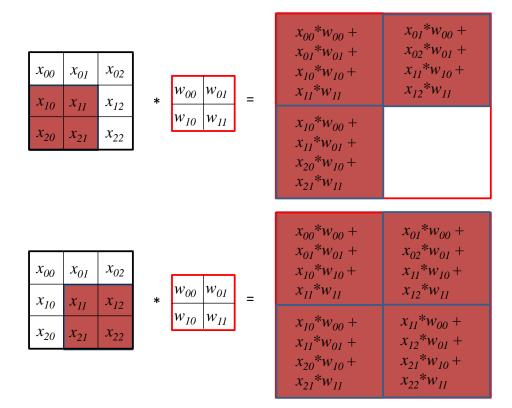
Take a moment to understand how the computation above is being done. We slide the 2x2 kernel matrix over our 3x3 image by a 1 pixel stride, and for every position, we compute the elementwise dot product to get a single element of the output matrix. Note that the  $2\times2$  filter matrix "sees" only a part of the input image in each stride.
