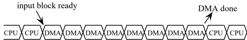
Figure 6.6. An input block is transferred all at once during burst mode DMA.
