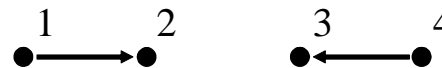
Fig. 3. Example failure scenario of BTSP. Node 1 has HP packets intended for Node 2. Node 4 has LP packets intended for Node 3. The four nodes can only hear their adjacent neighbors' transmissions. If Node 4 gains access first then it can suppress the HP stream from Node 1. As part of Node 4's contention, Node 3 sends a CTS that mutes Node 2. When Node 1 contends, Node 2 cannot respond. Node 1 considers the contention a failure, increases its contention window and contends again. The busy tone scheme cannot affect Node 4 and so Node 1 can only seize the channel if by chance its contention window expires between Node 4's transmissions.
