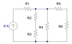
Current throught R4=  $\pm 2$  A (depending on direction assumed) Voltage across resistor R3 =  $\pm 6V$  (depending on direction assumed)
