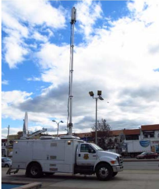
Fig. 24. Two COLTs in Long Beach. The one in the back is still being installed.
