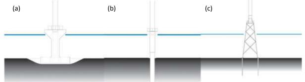
**Figure 1**. Illustrations of the three most common foundations used for offshore wind farms. (a) Concrete gravitation foundation, (b) steel monopile foundation and (c) steel jacket foundation. Illustrations modified from Hammar *et al.* (2010) with curtsy of Linus Hammar.
