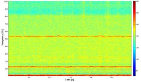
**Figure 9**. Spectrogram of 5-min recorded operational noise 160 m from a turbine at the Lillgrund wind farm. The tonal components are clearly visible below 1 kHz with 127 Hz being the strongest tone. The sliding effect is clearly visible for 533 Hz tone. The colour bar to the right shows the sound pressure in dB re 1 $\mu$ Pa.
