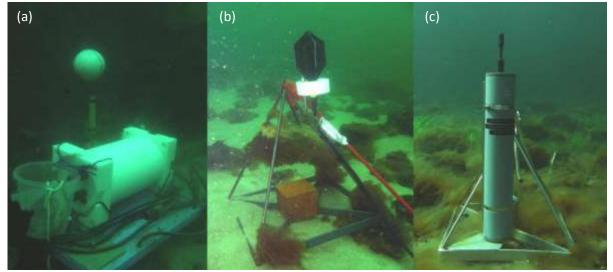
**Figure 3**. Acoustic sensors used in the studies. (a) Particle motion sensor developed and used in **PAPER IV**, (b) Brüel & Kjær 8101 hydrophone and (c) DSG-ocean hydrophone used in **PAPER V**. © Mathias H. Andersson.
