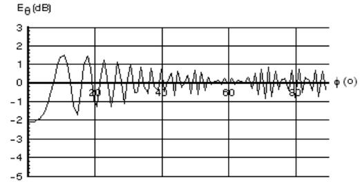
Fig. 5. Far field radiation pattern for a transmitter antenna height of 20 m and a distance of 100 m to the pylon axis at 100 MHz.
