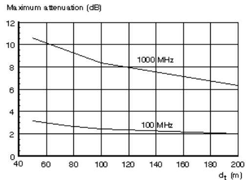
Fig. 11. Maximum attenuation as a function of transmitter antenna to obstacle distance  $d_t$ .
