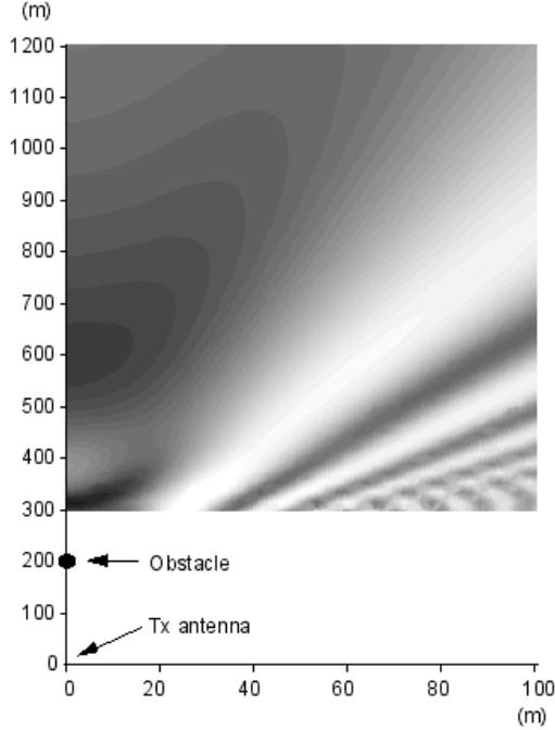
Fig. 7. Obstacle attenuation for  $d = 200$  m calculated using WIPL-D at 100 MHz.
