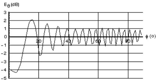
Fig. 2. Far field radiation pattern for a pylon axis distance of 50 m at 100 MHz.
