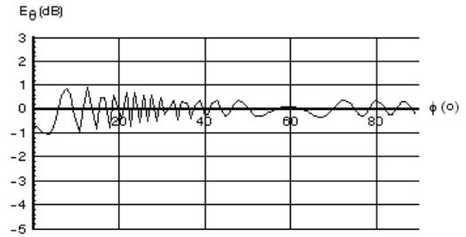
Fig. 4. Far field radiation pattern for a pylon axis distance of 200 m at 100 MHz.
