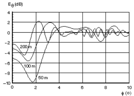
Fig. 12. Far field radiation pattern for transmitter antenna to pylon axis distances of 50, 100 and 200 m, at 1000 MHz.
