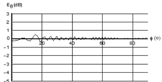
Fig. 6. Far field radiation pattern for a transmitter antenna height of 50 m and a distance of 100 m to the pylon axis at 100 MHz.
