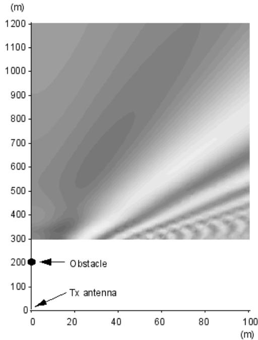
Fig. 9. Obstacle attenuation for  $d = 200$  m calculated using the Kirchhoff-Huygens formulation at 100 MHz.
