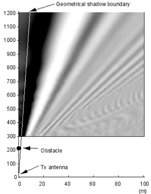
Fig. 10. Obstacle attenuation for  $d = 200$  m calculated using the Kirchhoff-Huygens formulation.
