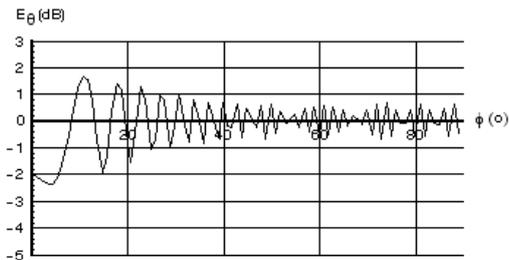
Fig. 3. Far field radiation pattern for a pylon axis distance of 100 m at 100 MHz.
