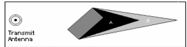
Figure 1.1 – Shadowed areas due to structures
