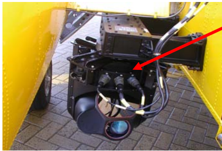
Fig 7 : TV and TI camera housing
