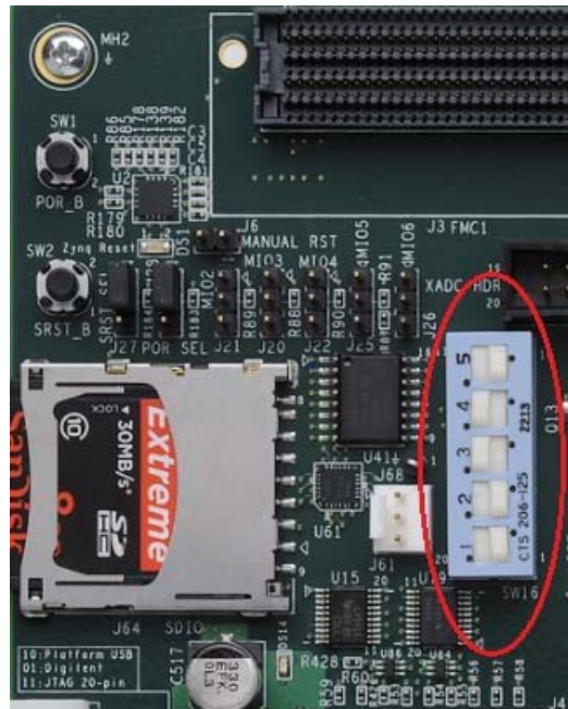
Figure 6-15: Jumper Settings for Booting Linux from SD Card
