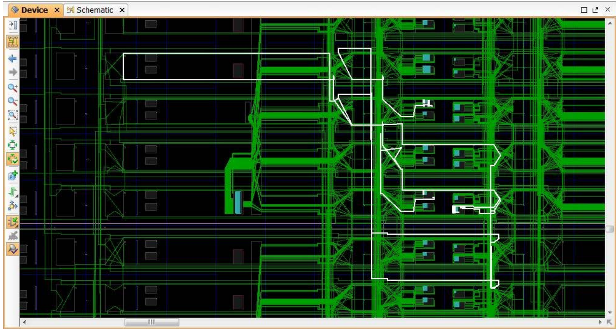
Figure 8: Displaying the Device Routing
