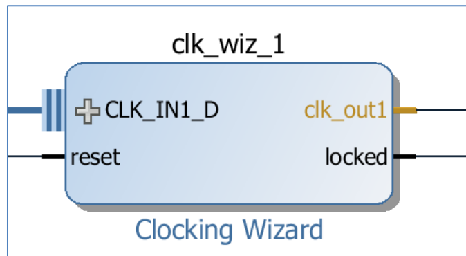
Figure 103: Analyzing the Clock Properties in IP Integrator
