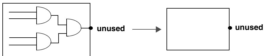
Figure 6-4 Minimizing Logic Driving an Unconnected Output Port
