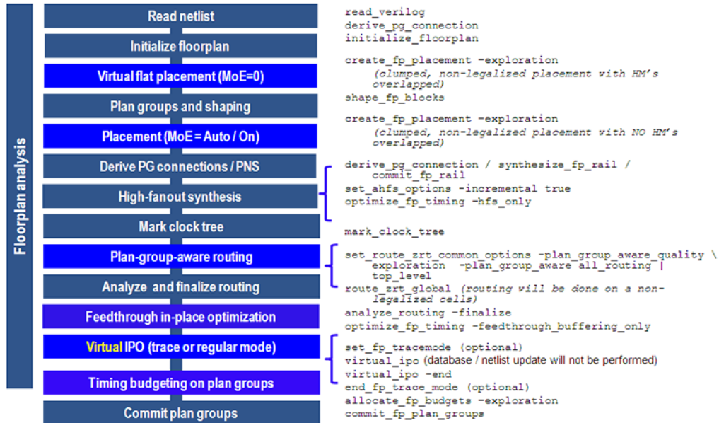
Figure 6-22 Timing-Driven Exploration Flow
