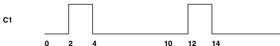
Figure 7-1 C1 Clock Waveform
