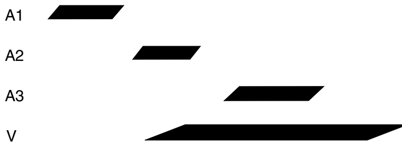
Figure 2-5 Multiple Aggressor Alignment
