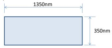
Where:  $C_{bottom} = 23 \text{ ff/}\mu^2$  and  $C_{sidewall} = 10 \text{ ff/}\mu$
