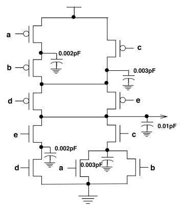
(a) Find the delay when (a b c d e) makes the following transitions: 0 0 0 0 0  $\Rightarrow$  0 0 0 1 1  $\Rightarrow$  0 0 0 0 1.
