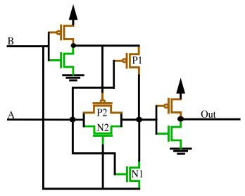
b)(6 pts) Give the minimum CMOS realization of an XNOR ( $f = \overline{a \oplus b} = ab + \overline{a}\overline{b}$ ). Assume the **un**complemented inputs a and b are available. Show your work.
