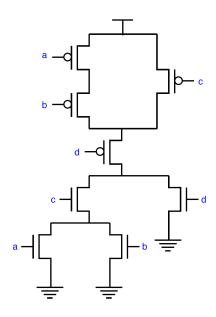
(a) Label the four inputs in the circuit below with the clock symbols CLK and CLKB (complement of CLK) so that the flop latches at the falling edge of the clock.
