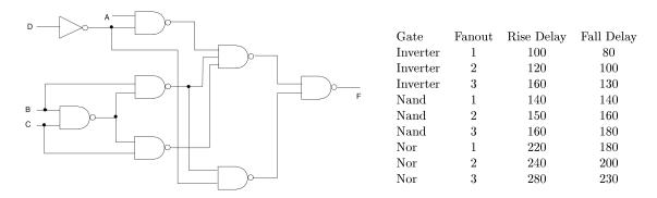
Find the longest functional paths from inputs D and C to F and give the rise and fall delays.
