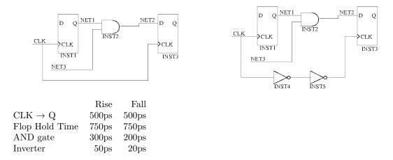
4. (a) Identify if there are any hold time problems from the source flops (G1, G2, G3 and G4) to G11 in the circuit below. If there are any, indicate by how much the hold time is violated and suggest a fix which minimizes the impact on the delay of the circuit. Use the delays from the table below.
