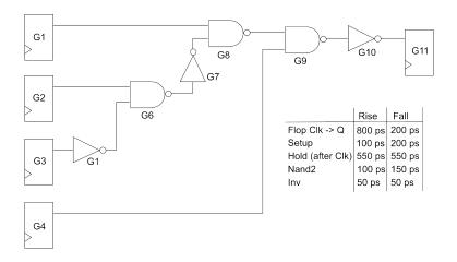
(b) What is the maximum frequency of operation after fixing any hold-time violation?
