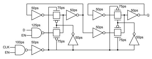
2. (a) Find the setup time, hold time and clock-to-Q delay of the pulse-flip-flop below.
