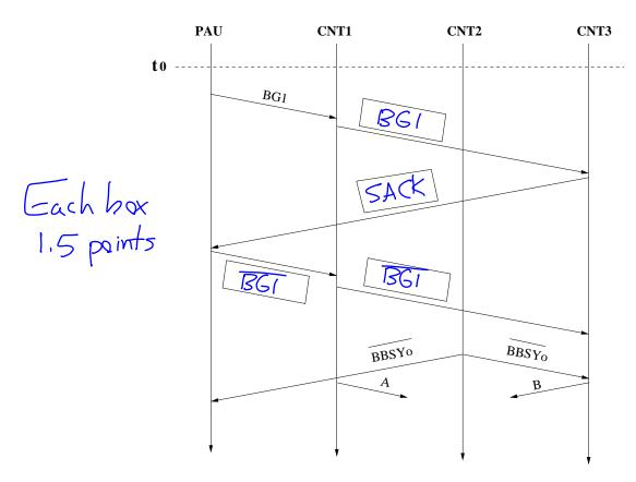
At t0, a bus master asserts BBSYo, allowing arbitration for the next bus cycle to begin. If you examine the entire timing diagram, can you tell which controller acquires the bus at t0?
