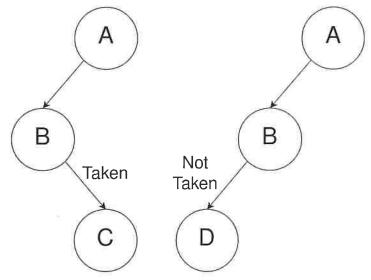
A Trace Cache element contains three basic blocks A,B,C, as shown, and the predictions for the branches terminating each block. The next time (at t-one) that the Trace Cache access corresponds to the starting address of A, the branch terminating B is predicted to fetch the block D, rather than C, as shown. In my implementation of the Trace Cache, what does the microarchitecture do with each block (A,B,C,D) at time t-one?
