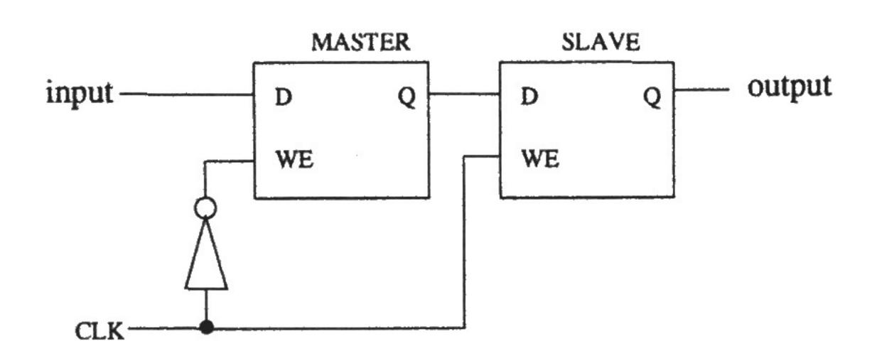
Note that the input value is visible at the output after the clock transitions from 0 to 1.
