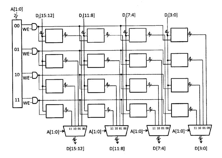
Part a: Unfortunately, the memory was wired by an engineering student from an un-named university, and he got the inputs to some of the muxes mixed up. That is, instead of the 4 bits from a memory cell going to the correct 4-bit input of the mux, the 4 bits all went to one of the other 4-bit sources of that mux. The result was, as you can imagine, a mess.
