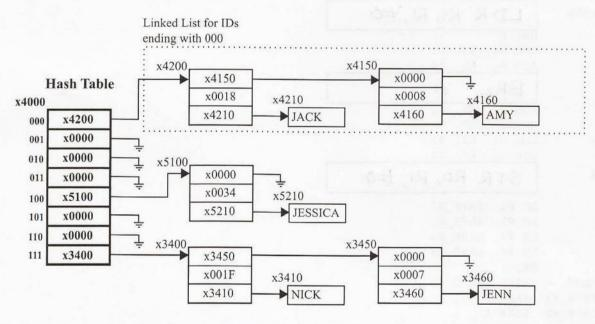
Actually, the data structure world does have names for this mechanism. The function used to determine which linked list is called a "hash function," and the table of pointers to the first element of each linked list is called a "hash table," but you don't need these names to solve the problem.
