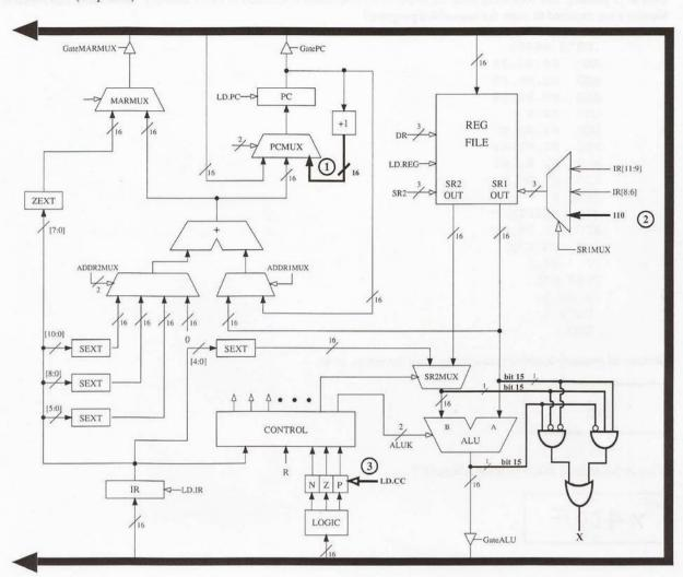
Part a. (6 points): Note that several of the lines (i.e., signals) in the LC-3 data path have been drawn in boldface. The line is designated by a boldface number 1,2,or 3. Not all instructions use all three lines. That is, some instructions would not function correctly if the line (i.e., signal) were removed.
