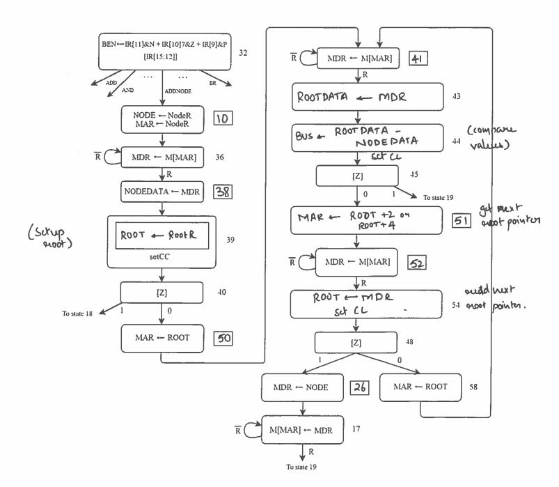
Part c (7 points): To handle the new micro-branches, we need to augment the microsequencer with an additional control signal ECS (Extra Control Signal).
