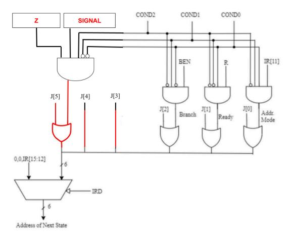
Part c (4 points): Modify the microsequencer below with the correct control logic:
