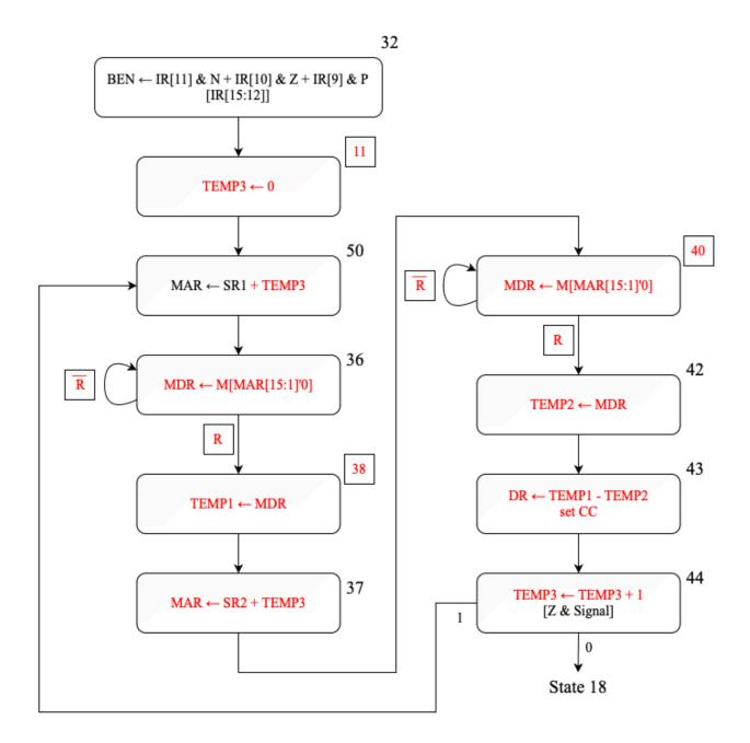
Part a (10 points): Complete the state machine below:
