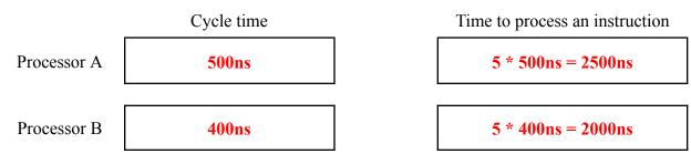
**Part b (4 points):** A program that has no control instructions and no stalls due to dependencies is executed by each processor. The number of instructions in the program is large. What is the average number of instructions executed per ns for each processor?
