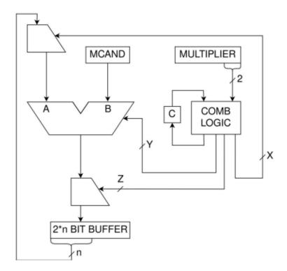
For an instance of Booth's Algorithm, bits [13:8] of the multiplier are 011101. These are used in iterations 5, 6, and 7.
