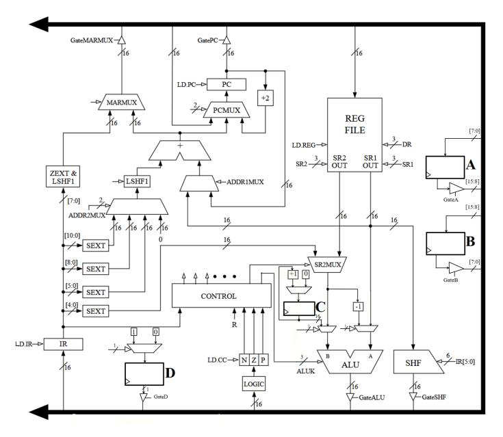
**Part d (6 points):** This new instruction involved changes to the microsequencer. A new control signal, COND2, has been added to the microsequencer. Complete all missing wires and determine the signal X.
