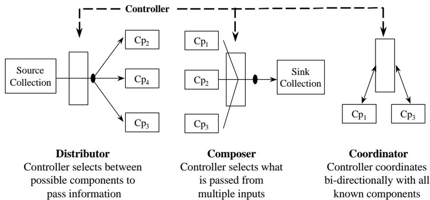
**Figure 1: Functional Models of a Controller Integration Element**
