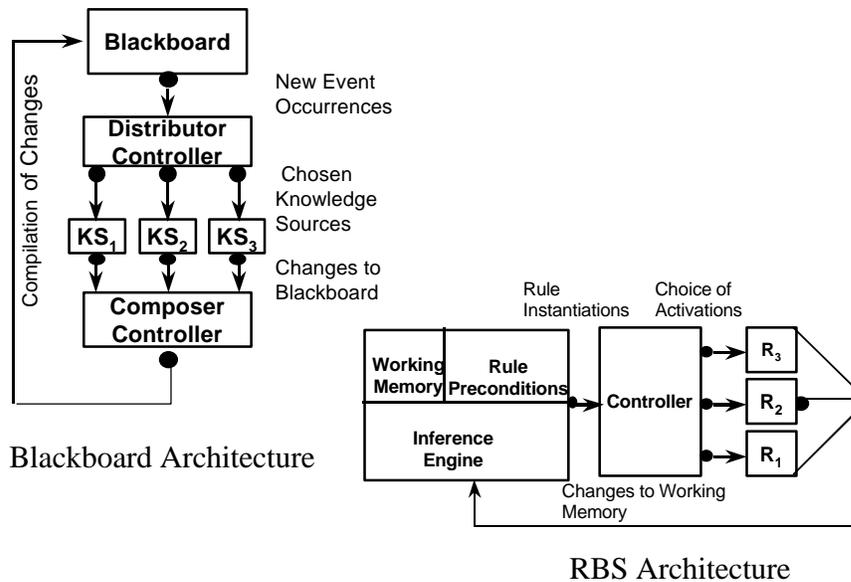
**Figure 2: The Blackboard & Rule-based System Architectures**
