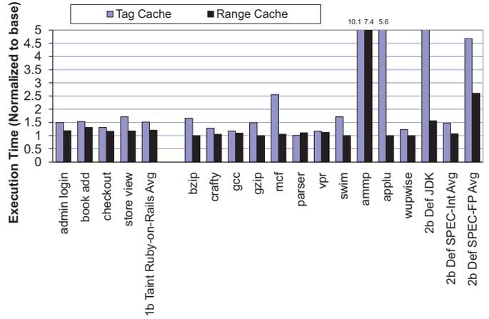
(a) Performance for 1-bit (Taint tracking on Ruby-on-Rails Application) and 2-bit (Definedness tracking for SPEC apps and JDK).
