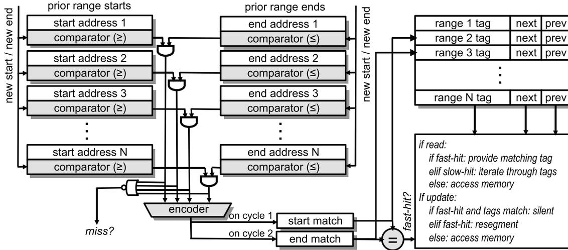
Figure 2: Range Cache Architecture: The first pipeline stage matches the start and end points of the new range, while the second stage is a state machine that performs tag lookup and decides on the aggregated range entry to be written back.
