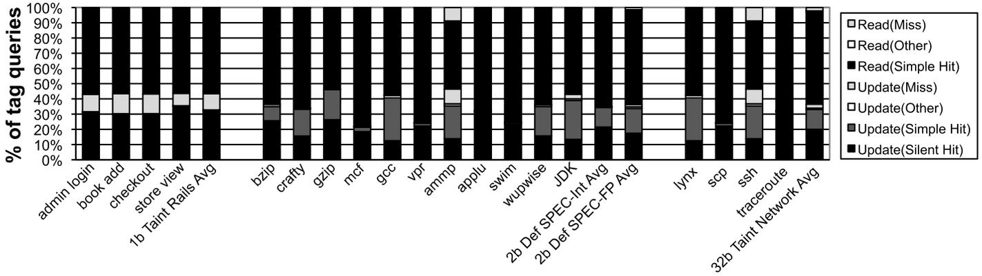
Figure 5: The relative proportion of various range queries for Dataflow Tracking. The SPEC applications (bzip through wupwise) are run with the definedness tracking tool, while the Ruby applications (admin login through store view) and network applications (lynx through traceroute) are run with network input taint tracking. The vast majority of accesses fall into “fast” categories where the updates are simple and the reads are hits to a single range.
