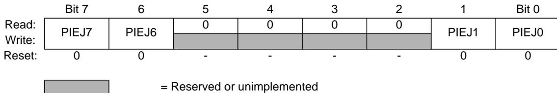
**Figure 3-44 Port J Interrupt Enable Register (PIEJ)**
