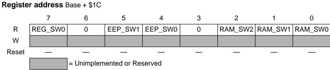
**Figure 3-8 Memory Size Register Zero**
