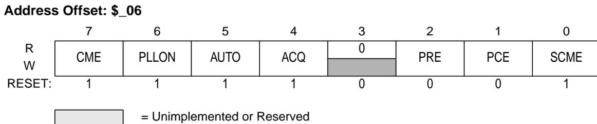
**Figure 3-7 CRG PLL Control Register (PLLCTL)**
