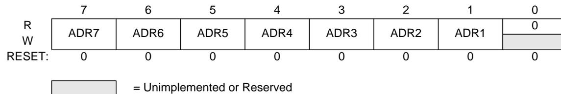
**Figure 3-1 IIC Bus Address Register (IBAD)**
