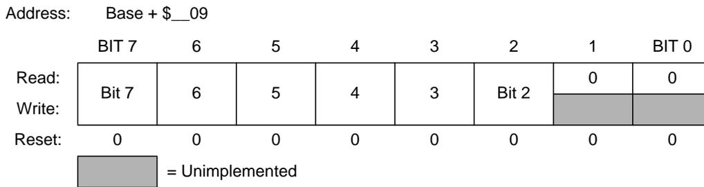
**Figure 3-8 Data Direction Register E (DDRE)**
