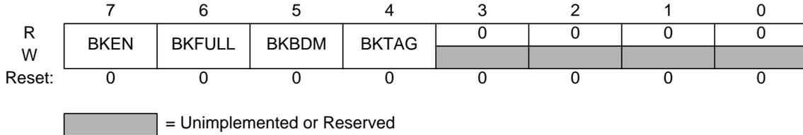
**Figure 3-2 Breakpoint Control Register 0 (BKPCT0)**
