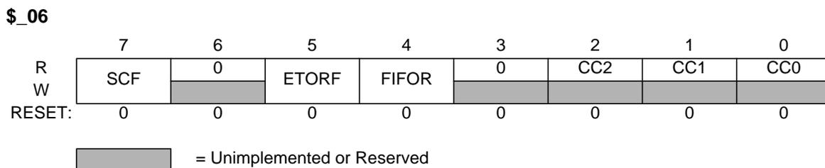
**Figure 3-7 ATD Status Register 0 (ATDSTAT0)**
