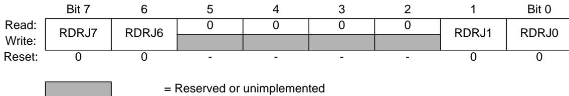
**Figure 3-41 Port J Reduced Drive Register (RDRJ)**
