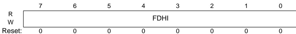
**Figure 3-12 Flash Data High Register (FDATAHI)**
