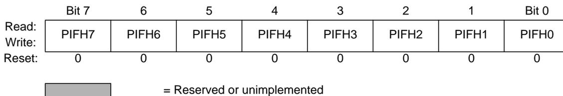
**Figure 3-37 Port H Interrupt Flag Register (PIFH)**
