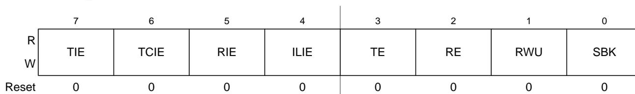
Figure 1-5. SCI Control Register 2 (SCICR2)
