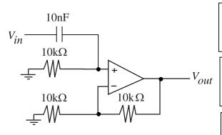
**Part a)** What is the gain at f much less than 100 Hz? C is open, gain is 0
