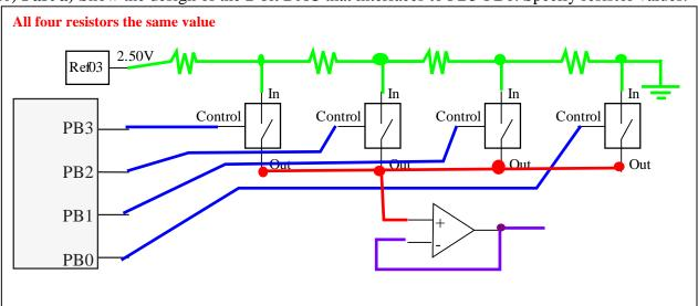
(5) Part b) Write the C function taking a 2-bit data input, setting the DAC to 0, 0.625, 1.25, or 1.875V.
